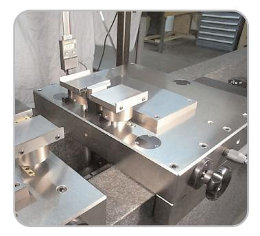
Robust air bearing slide with vertical setting feature and hardened stage surfaces. Air bearing slide features a manual drive with fine adjustment and lock to hold position.
