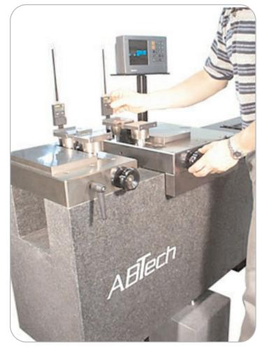
The setting master features user friendly position control adjustments for both vertical and horizontal setting. The unique air bearing slide and manual drive combine for ultra-smooth horizontal motion.
