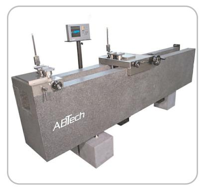
ABTech, Inc. has developed a Setting Master using a natural granite base and air bearing slide for set up of I.D./O.D. beam type gages such as Federal Products Series 980. The granite base in combination with the air bearing slide ensures a stable, and low maintenance gage.
