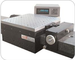
ABTech, Inc's precision air bearing linear slides offer a high accuracy solution to the most demanding optical radius inspection applications. The fully captured air bearing carriage offers friction free motion while the natural granite rail provides a stable and straight guide way.
